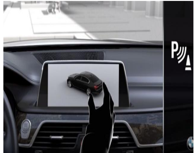
Fig.7. Change rear- view camera angle: Create a circle with your thumb and fore finger.
