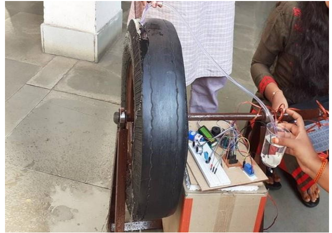
Fig 6: Detection of Tyre Temperature and Indication with Automatic Water/N 2 Spray
