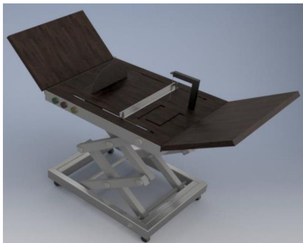
Fig. 2. 3D design model for semi-automatic acrylic cutter and bending machine
