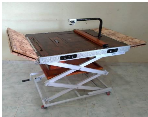
Fig. 4. Fabricated semi-automatic acrylic cutter and bending machine
