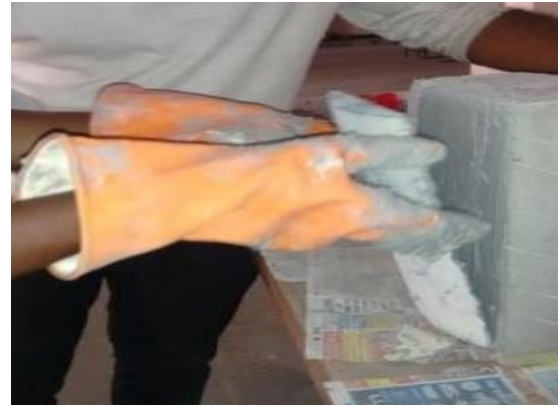
Fig. 3. Bonding of precast segments
