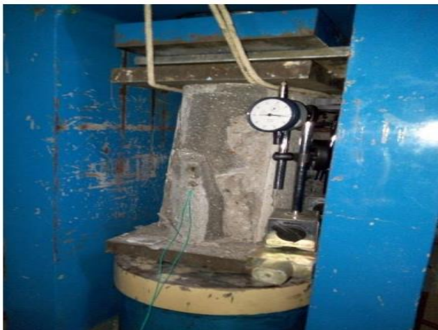
Fig. 6. Test set up in compression testing machine
