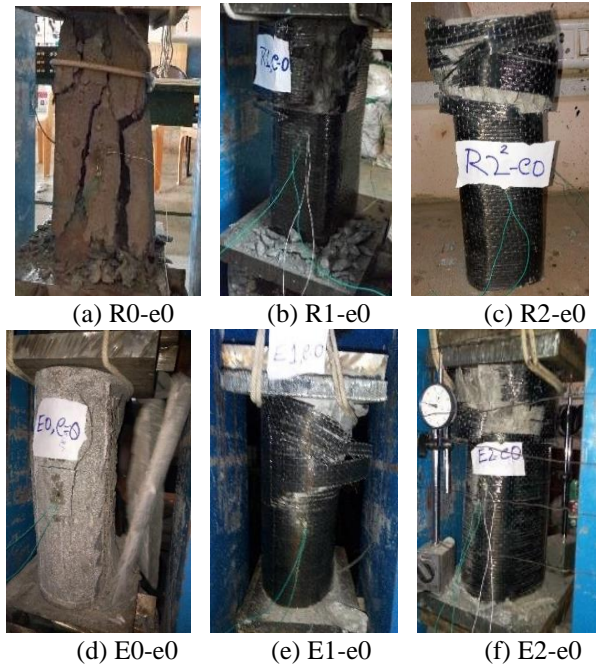
Fig. 8. Modes of failure of concentrically loaded specimens
