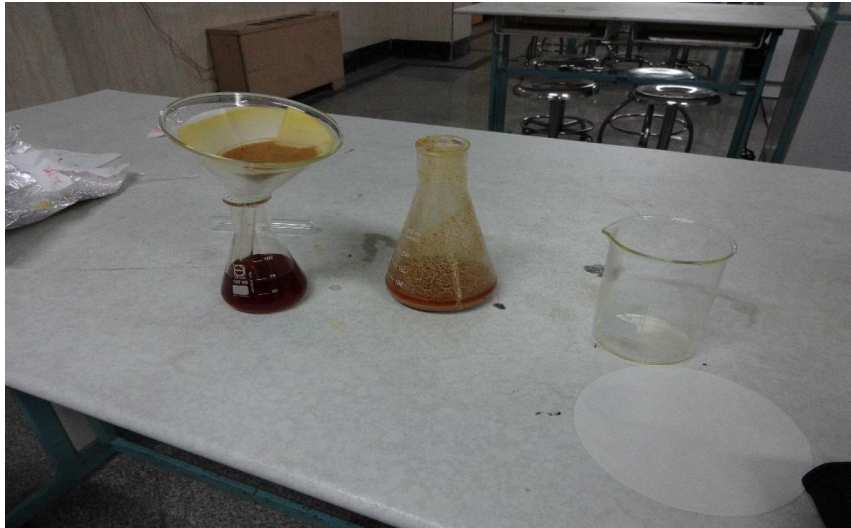
Fig. 4: Extraction phase. The combination of ginger and alcohol gets filtered by use of funnel and filter paper to get the pure solution with no solid inside.
