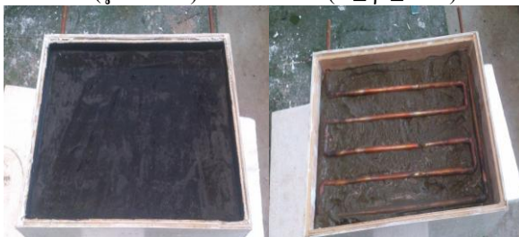
Fig. 1. A photograph of one of the solar water heaters.
