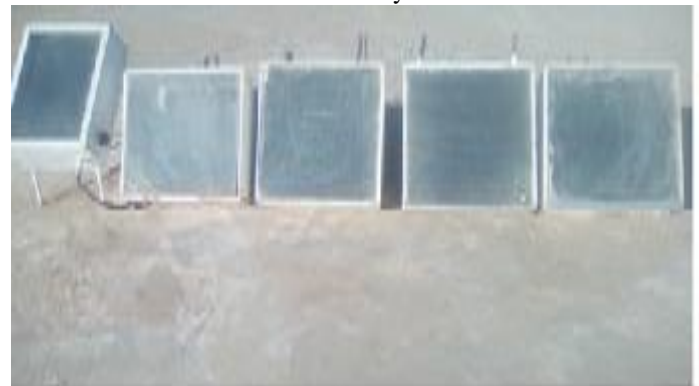
Fig 2. A photograph of the five solar water heaters prototypes on site.
