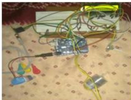
Fig: Syringe connected to DC motor, ECG sensors, temperature sensor, pulse sensors connected to arduino
