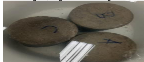
Fig. 7. Water Absorption test.
