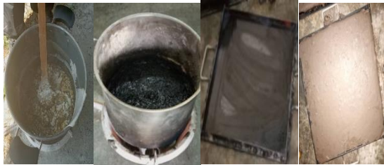
Fig. 3. Melting of PET waste Fig.4. PET waste & sand mixture Fig. 5. Floor tile mold Fig.6. Plastic floor tile produced.
