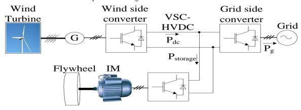
Fig1. VSC-HVDC transmission system
