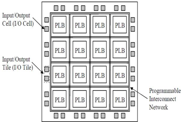
Figure 1: Typical FPGA Architecture
