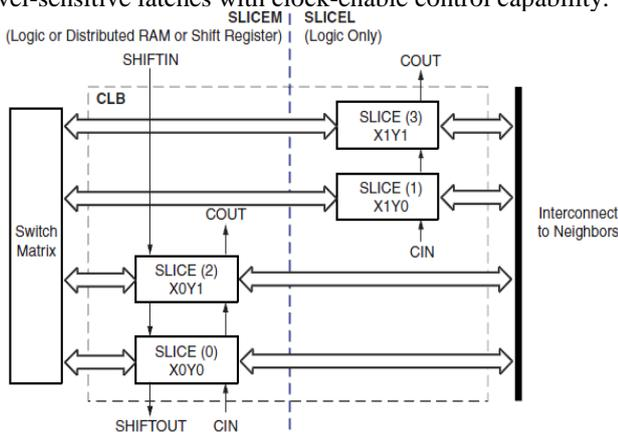
Figure 2: Arrangement of Slices within the CLB
