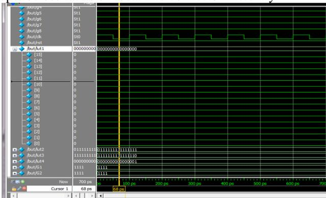
Figure 8: stuck-at-0 fault on 16<sup>th</sup> cell
