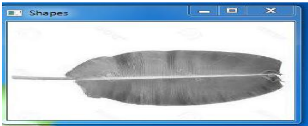
Fig 4: Converting the affected image to the blur image by Using Gaussian blur algorithm.
