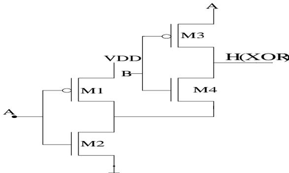
Fig.14T XOR logic circuit
