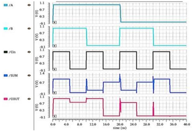
Fig. 5(a) Simulation input-output waveforms of the N17T FA  $V_{DD} = 1V$
