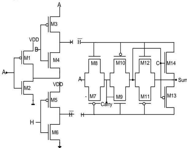
Fig. 4(b) N14T FA circuit
