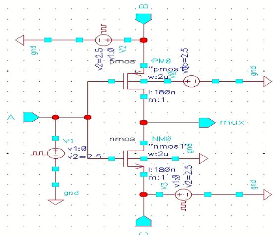
Fig. 3 Schematic diagram of 2T MUX logic circuit
