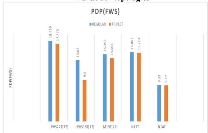
**Fig.16. PDP of regular and triplet design 4-bit RCA Fulladdertopologies**
