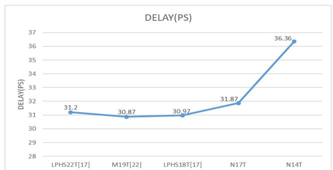
Fig. 7 Comparative delay analysis of five adder topologies
