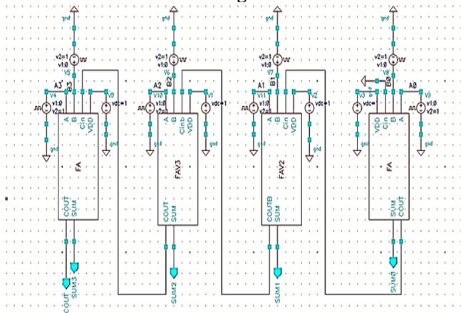
**Fig. 13(b) Schematic diagram of proposed 4-bit RCA triplet design**
