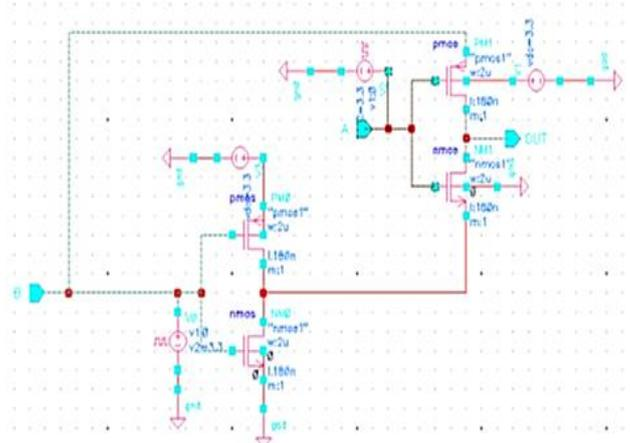
Fig. 2 Schematic diagram of 4T XOR logic circuit
