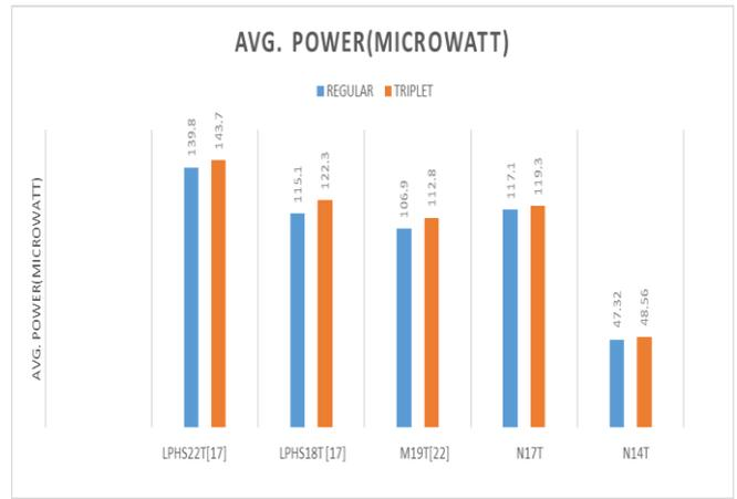
**Fig. 14. Avg. Power of regular and triplet design 4-bit RCA Fulladder topologies**
