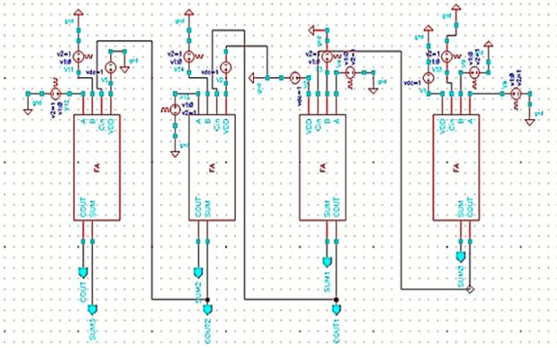
**Fig. 13(a) Schematic diagram of 4-bit RCA regular design**
