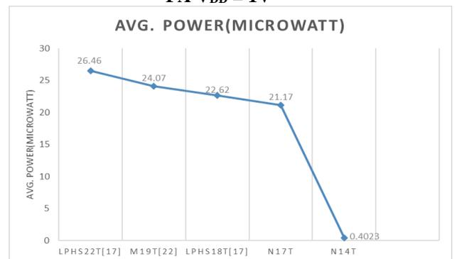
Fig. 6 Comparative Avg. power analysis of five adder topologies
