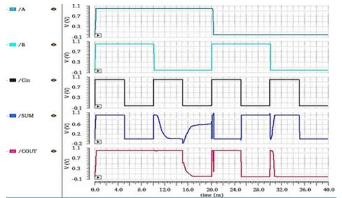
Fig. 5(b) Simulation input-output waveforms of the N14T FA  $V_{DD} = 1V$
