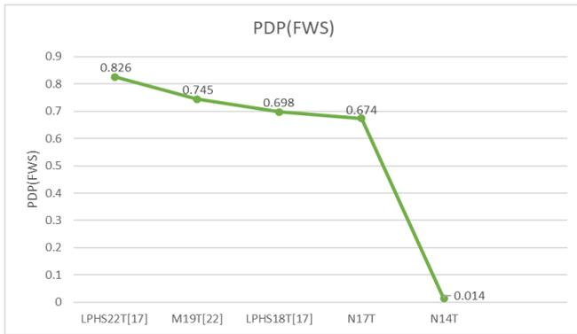
**Fig. 8 Comparative PDP analysis of five adder topologies**
