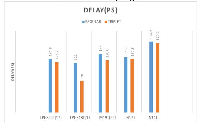
**Fig. 15. Delay of regular and triplet design 4-bit RCA Fulladder topologies**
