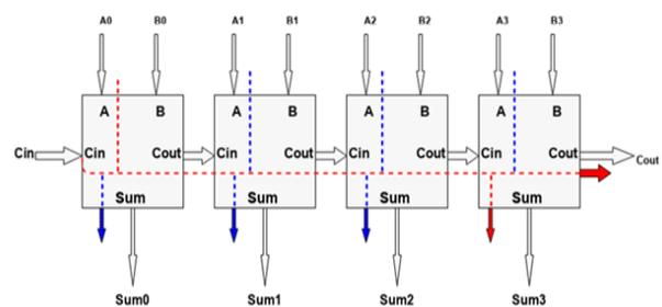
**Fig. 11 4-bit RCA regular design [17]**
