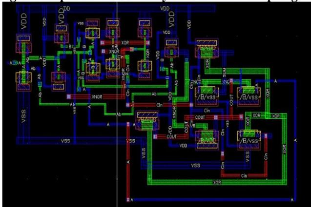
**Fig.9(a) Layout of N17T adder**
