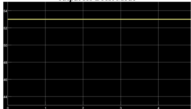
Figure.3 (b). Simulation result for 24V input to 53V dc output for Boost Mode
