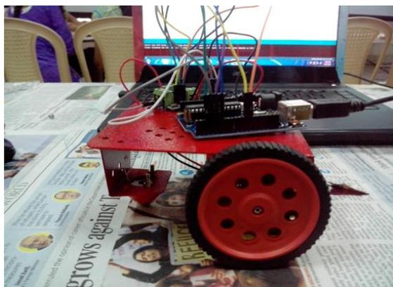
Fig. 5 Prototype of vision controlled robot
