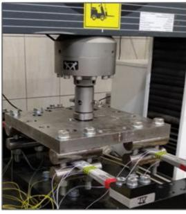
Figure 2. Tests on a bench for bending metal levers
