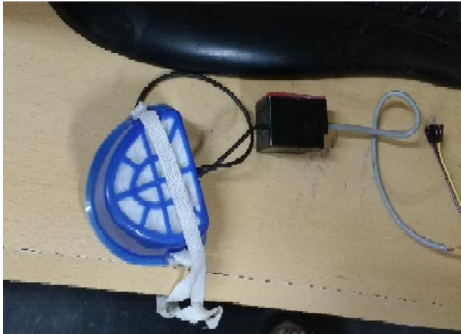
Fig.6 Alarm signal device
