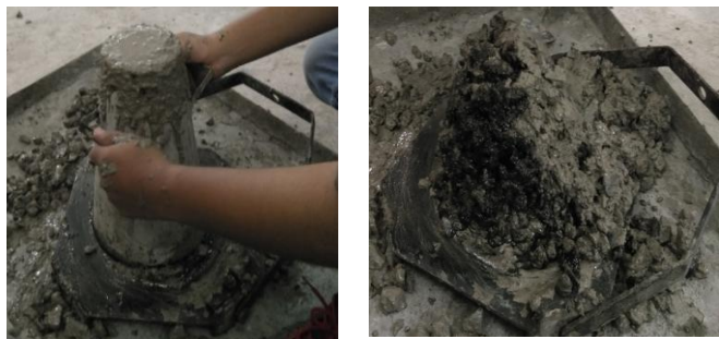
Fig. 4. Slump test and behaviour of slump
