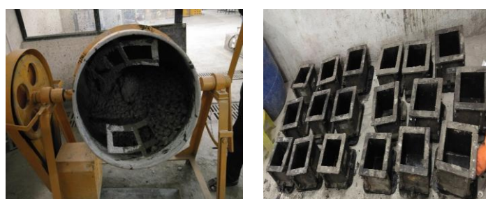
Fig. 2 Mixing of geopolymer concrete and preparation of moulds for casting
