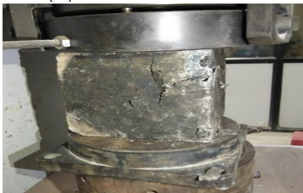
Fig. 5 GGBS mixed geopolymer concrete compressive strength test setup
