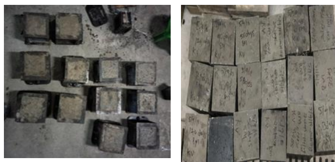
Fig. 3 Casting and curing under ambient temperature of GGBS mixed geopolymer concrete
