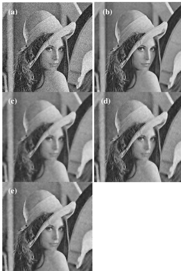
Fig (2): a)Noisy image with \sigma=20 , image denoised by b)WT c)WF d)GFMT e)Proposed method
