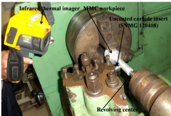
Fig. 3. Turning setup of the MMC.
