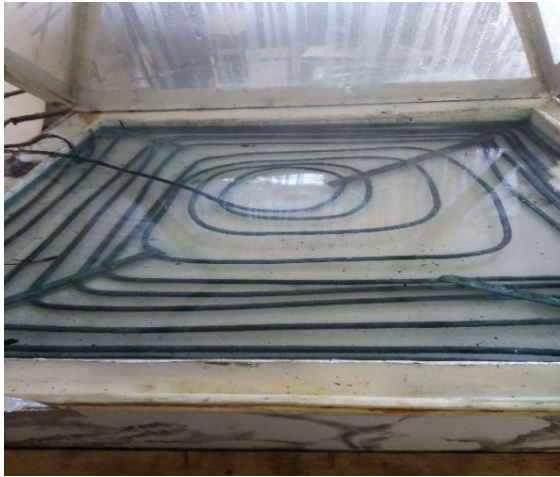
Fig. 4. The new condenser.
