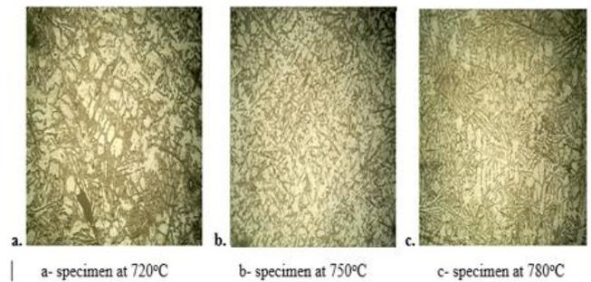
**Fig. 14: Microstructure of a sand cast Al metal composite with 2% of copper.**
