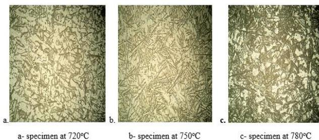
**Fig. 13: Microstructure of a sand cast Al metal composite with 0% of copper.**
