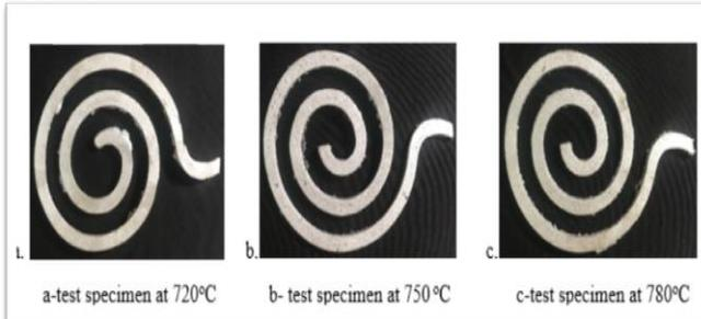
**Fig. 12: Specimen at 720, 750 and 780°C for 4% Copper**
