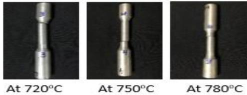
**Fig. 7: Tensile test specimen for 4% Cu**
