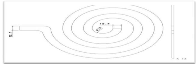
**Fig. 9: - Single spiral of 3.18mm thick, 12.7mm width and 940mm length**
