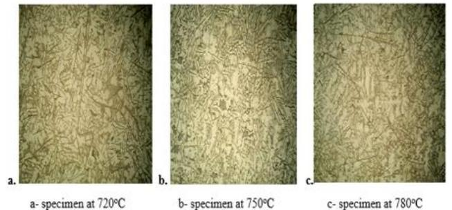
**Fig. 15: Microstructure of a sand cast Al metal composite with 4% of copper.**
