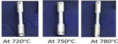
b. Specimen After Testing
