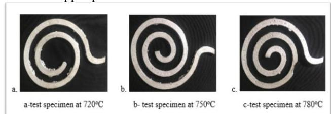
**Fig. 11: Specimen at 720, 750 and 780°C for 2% Copper**
