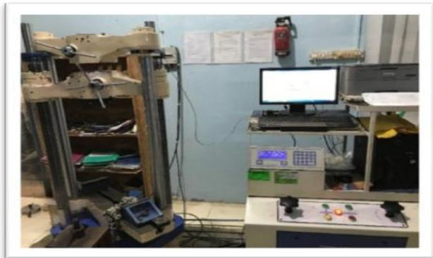
**Fig. 1: Universal Testing Machine**
