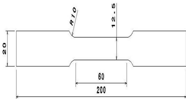
**Fig. 2: Schematic illustration of tensile test**
