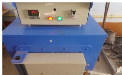
Fig. 5 Muffle Furnace for B 4 C particulate preheating up to 300°C.
