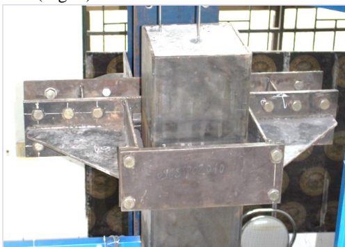
Fig. 10. Details of column anchor
