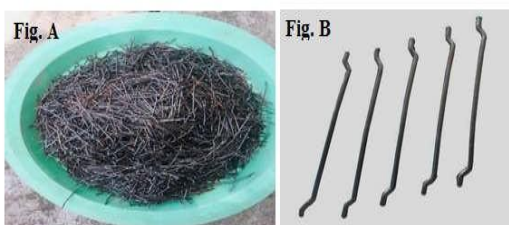
Hooked Steel Fibers used with Random orientation in Reinforced concrete
