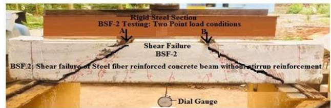
Shear Mode of failure in BSF2 beam using steel fiber concrete
