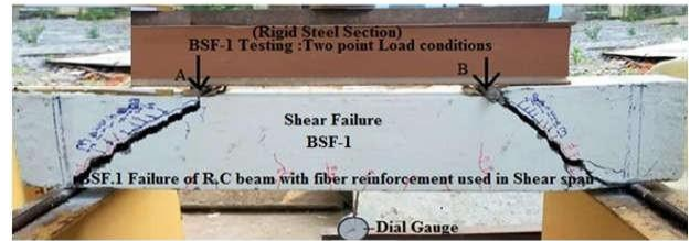
Shear mode of failure in Beam:BSF 1
