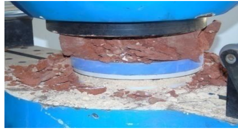
Figure-3: Compression test on UTM
