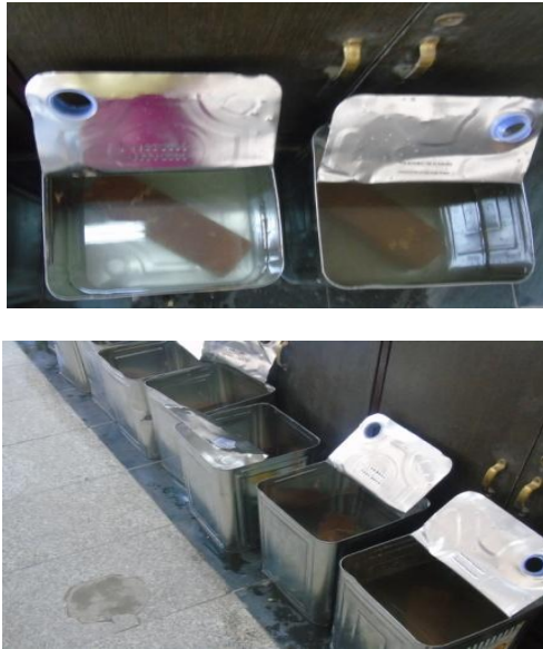
Figure-2: Water Absorption of bricks
