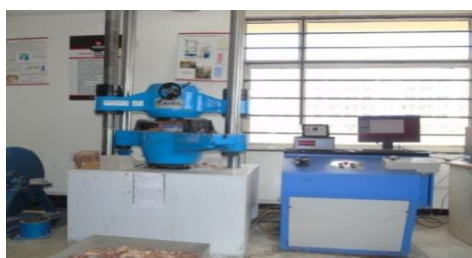
Figure-3 below shows compressive strength test on Universal testing machine.
