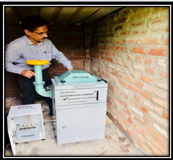
Figure- 8: Ambient air quality of both rooms and outside these rooms was monitored using RDS (Respirable Dust Sampler) for 48 hours.
