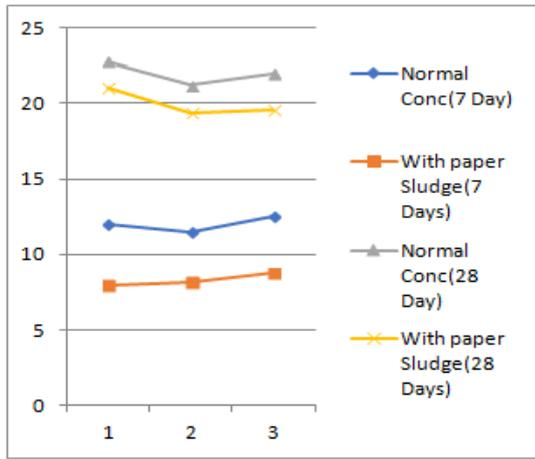
Figure 1: Concrete behaviour with or without sludge
