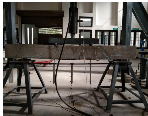
Figure 12. shows b3 with flexure and shear tension failure
