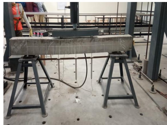
Figure 11. shows b2 with flexure and diagonal failure
