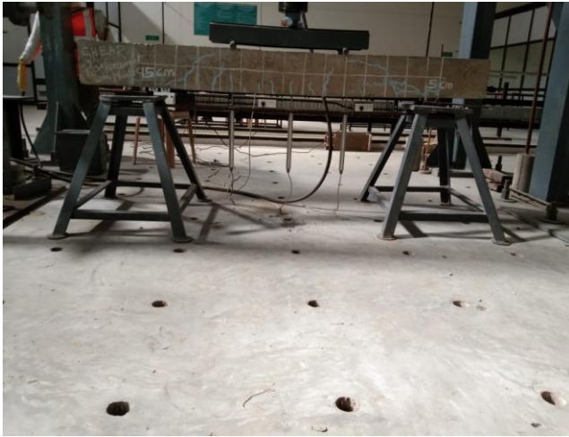
Figure 13. shows b4 with flexure and shear compression failure
