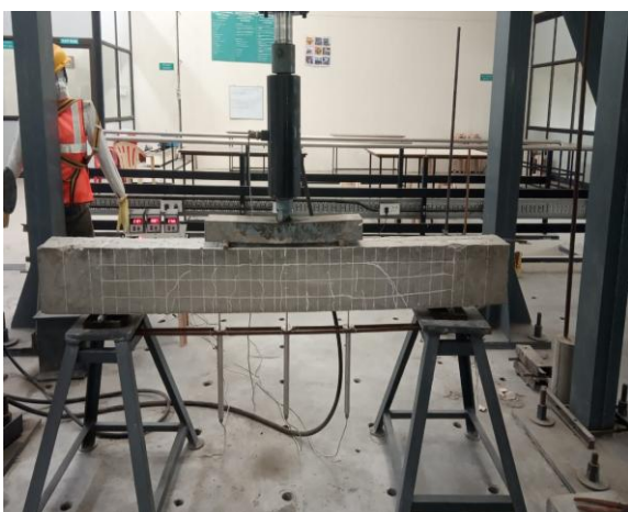
Figure 10. shows b1 with flexure and diagonal failure
