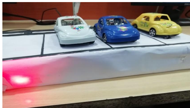
Fig. 3. Working model representing parking slot is occupied
