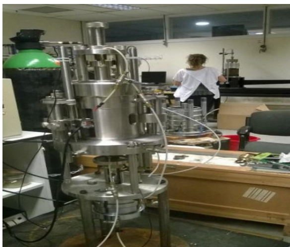
Fig 5: Controlled suction in a triaxial apparatus
