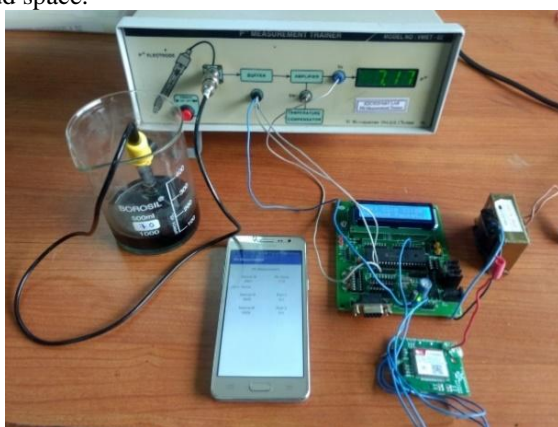
Fig. 5 Hardware Configuration of Wireless Sensor Network based monitoring of Water Quality
