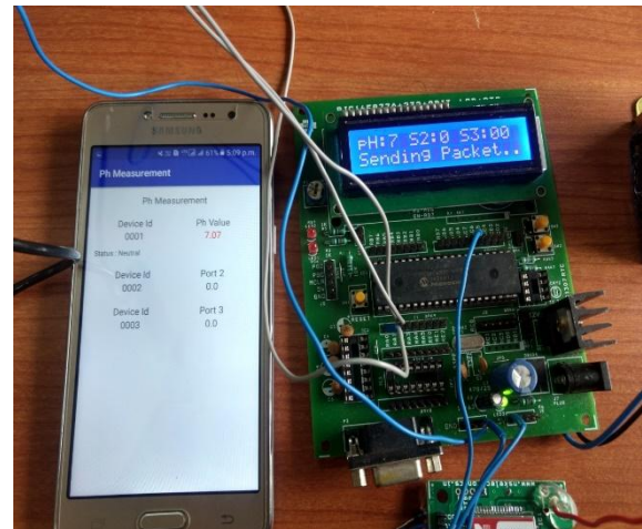
Fig.6 Software Configuration of Wireless Sensor Network based monitoring of Water Quality
