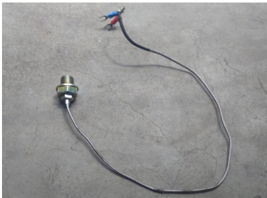
Fig 2.2 Temperature sensor inserted in drainage port.
