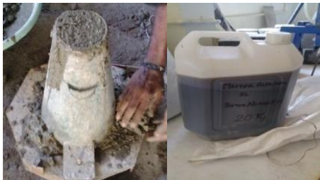
Pic 2. Workability test and superplasticizer Glenium51
