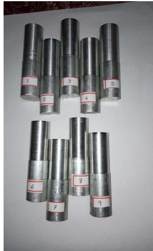
Fig. 3. Specimens after Turning in CNC lathe.
