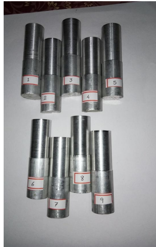
Fig. 3. Specimens after Turning in CNC lathe.
