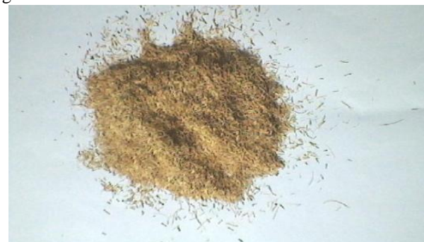
Fig. 1. Chopped Fiber after Chemical Treatment
