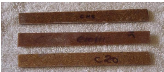
Fig. 3. Flexure test specimen
