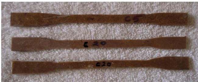
Fig. 2. Tension Test specimen
