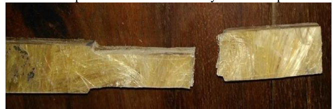
Fig. 8. Specimen after tensile test
