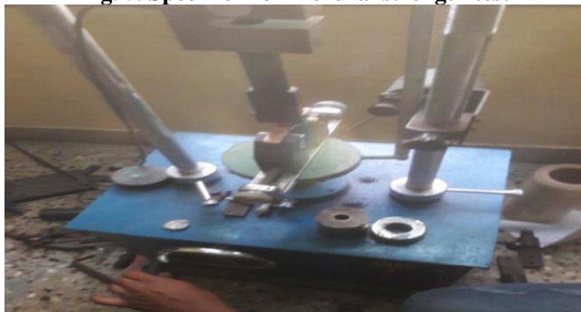
Fig. 6. Flexural strength test setup
