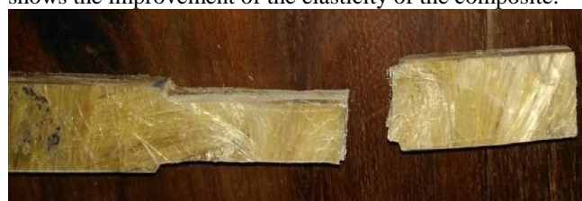
Fig. 8. Specimen after tensile test
