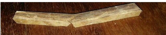
Fig. 12. Specimen after flexural strength test
