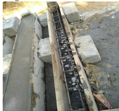
Fig. 4 Specimen with aerocon blocks
