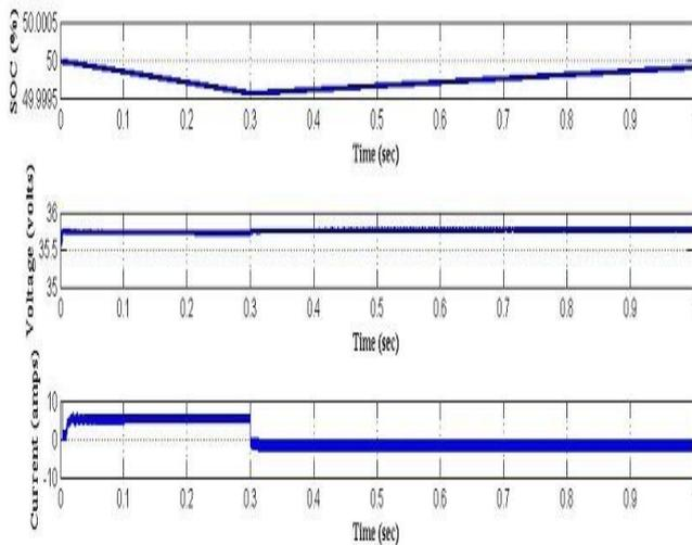
**Fig. 16. Simulation Result of Battery Voltage = 35.75V, current = 4.7A, SOC = 50%**
