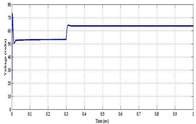
**Fig.15. Boost Voltage supplied to load  $V_{Boost} = 63.54$  V**
