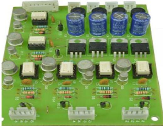
Fig. 2. TLP 250 in bridge rectifier
