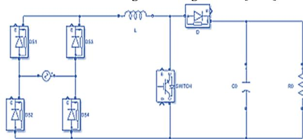
Fig. 1. Conventional PFC Rectifier
