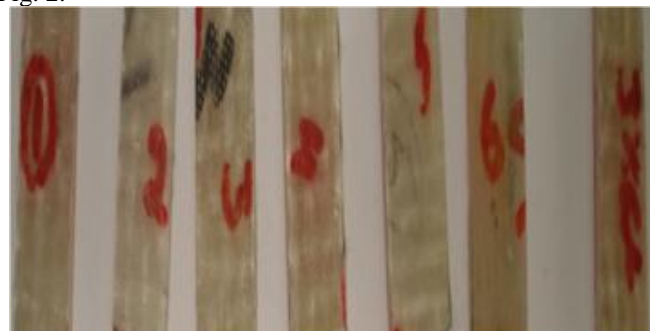
Fig.2. Wear specimens (1.5, 2.5 and, 3.5 wt%) reinforced with Halloysite HNT nano clay composite.
