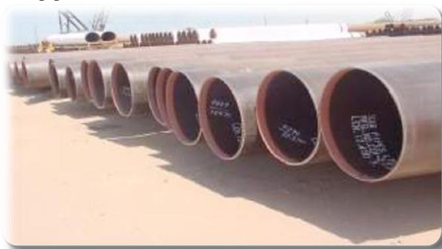
Fig. 5. Internal Plastic Coated Tubing (Courtesy: www.rigzone.com)
