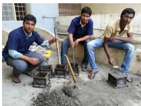
Fig:8 Casting of moulds
