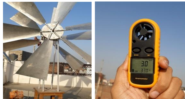
Fig. 2(a) Side view of real dual rotor assembly, (b) Anemometer wind speed and temperature measuring instrument.
