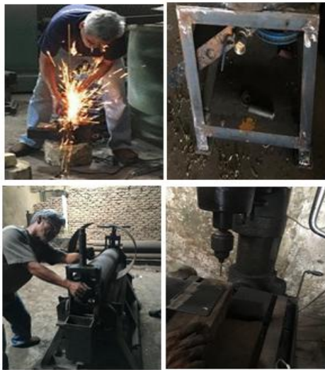
Figure 8. Manufacture of Cilembu Sweet Potato Cleaning Machine
