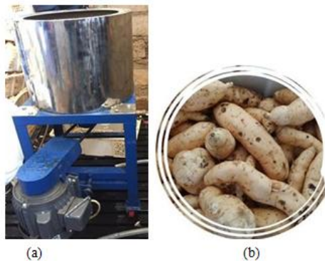
Figure 9. (a) Cilembu sweet potato cleaning machine (b) Cilembu sweet potato had cleaned
