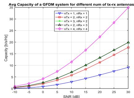
Fig. 6. Variation of capacity with respect to SNR
