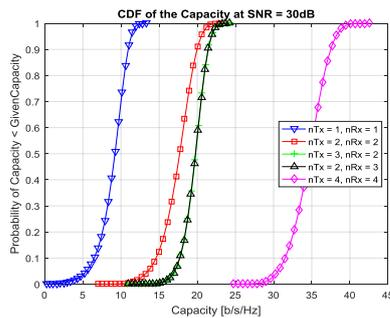
**Fig. 7 Probability of capacity curve at SNR=30dB**
