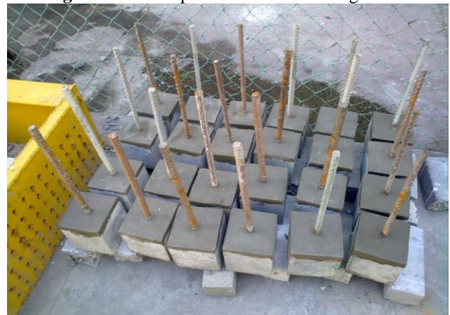
Fig. 5.Pull out Specimens after Cement Capping.
