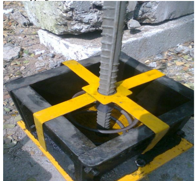
Fig. 4.Mould setup used for Bond Strength Test
