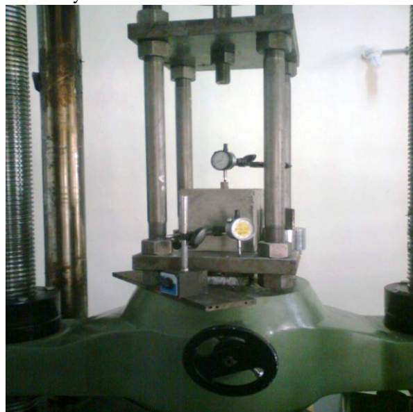
Fig. 7.Experimental Arrangement of Pull out experiment
