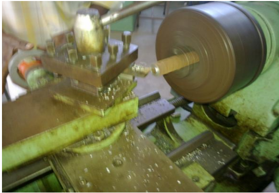
Fig. 1.Facing Process of Rebar in Progress
