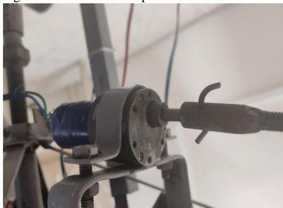
Fig. 12. Geared stepper motor
