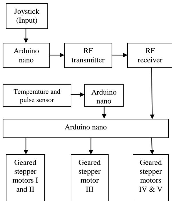
Fig. 3. Block diagram of proposed system
