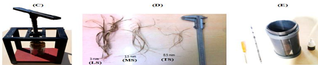
Fig. 2. The tools used for Samples preparation: compression tool(C), different size of esparto-fibers measured by a Calliper. (D), steel rods and Gabari (E).
