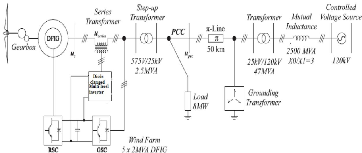
Fig 6 :Neutral clamped inverter base test grid
