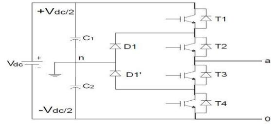
Fig 5: diode clamped MLI
