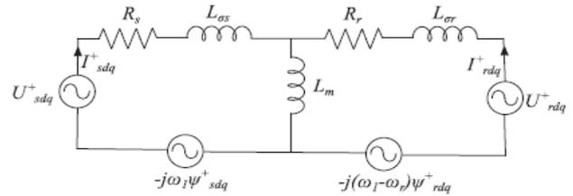
Fig 2. circuit representation of wound rotor machine
