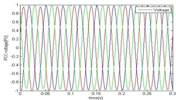
Figure(o): PCC voltage without compensation
