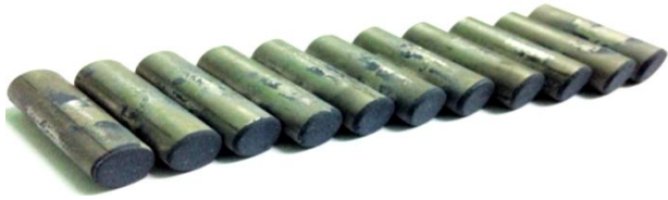
Figure 1. Plasma sprayed composite (Al 2 O 3 + 13% TiO 2 ) samples
