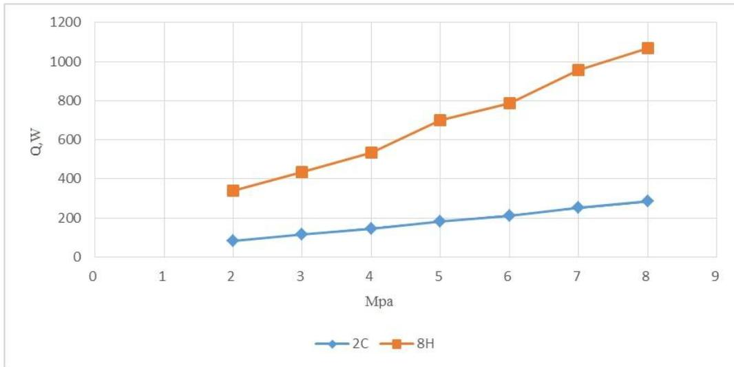
**Fig. 7: The dependence of the cooling power ( $Q_c$ ) on the pressure ( $P$ ), when using types 2C and 8H cold generators**
