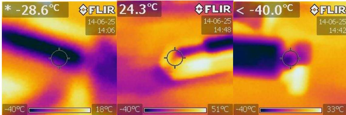
Fig. 3: Images of the temperature field at the cold outlet of the vortex tube, obtained by means of a thermal imager.
