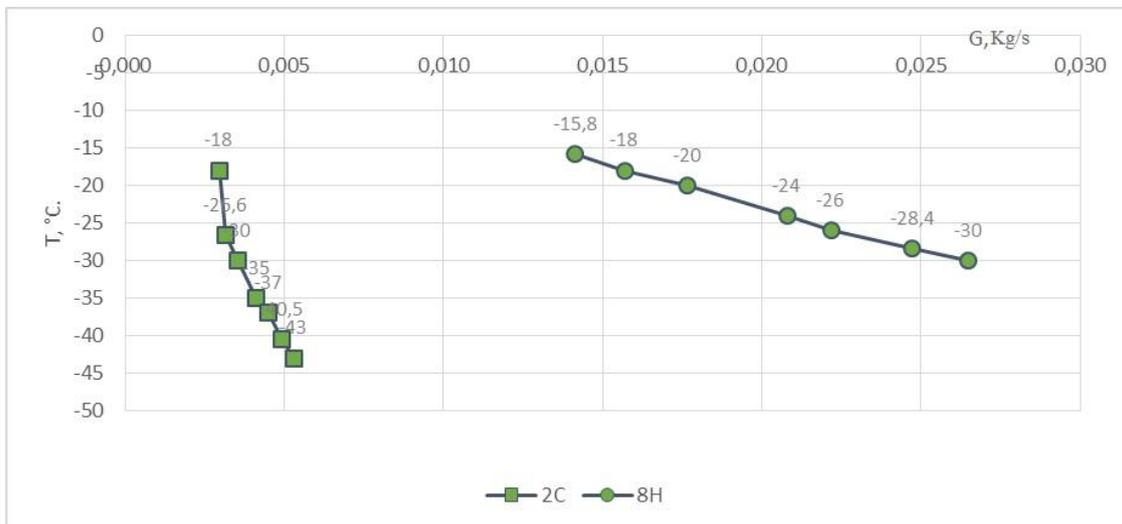
Fig. 6: Temperature ( $t_c$ ) dependence on the type of cold fraction generator for generators of 2C and 8H types.
