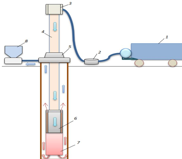
**Fig. 8: Schematic diagram of air flow at the location of the vortex tube above the core barrel.**
