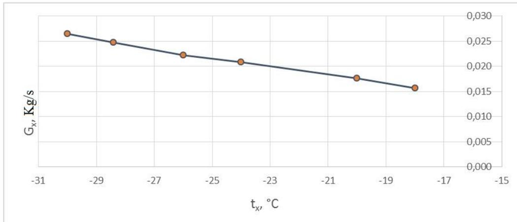
Fig. 5: The dependence of the cold flow temperature ( $t_x$ ) on the air flow rate ( $G_x$ ), when using the 8H-type cold generator.
