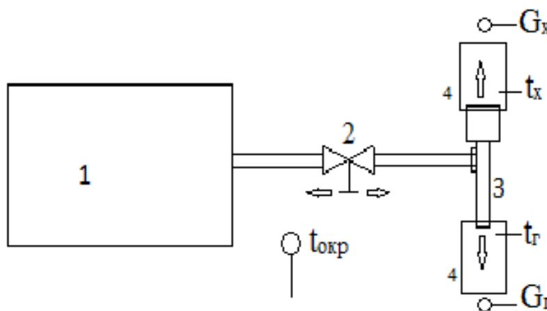
**Fig. 2: Schematic diagram of experimental installation with vortex tube.**
