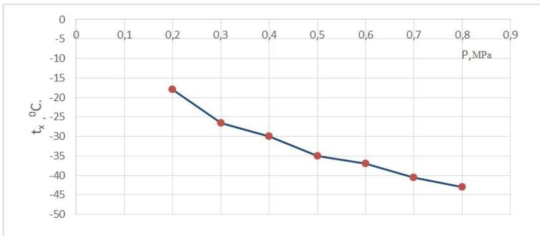
Fig. 4: The dependence of the temperature change (t) of the cold flow on the pressure (P), using the 2C-type cold generator.
