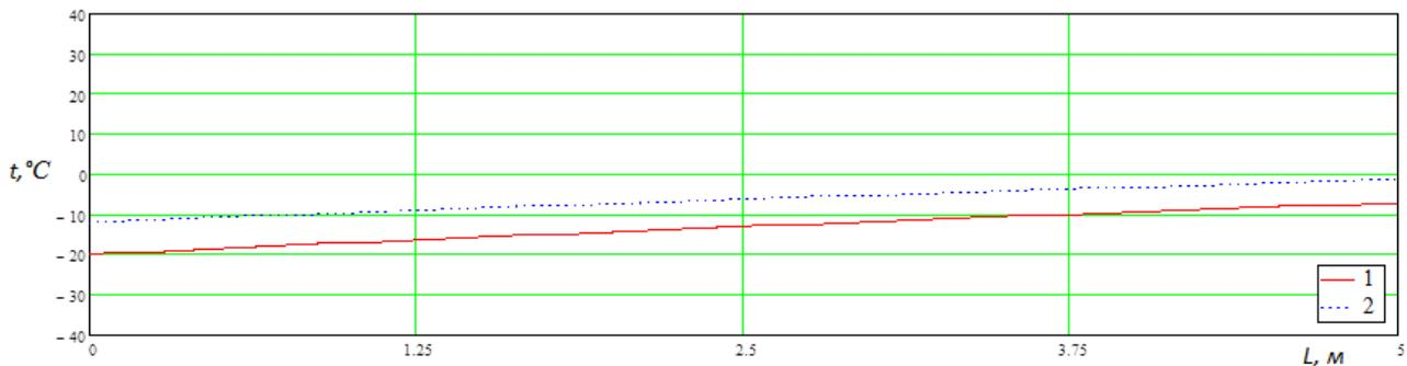
Fig.9: Temperature distribution when installing a vortex tube into the tool string above the core barrel: 1 – in the core barrel; 2 – in the annular channel.
