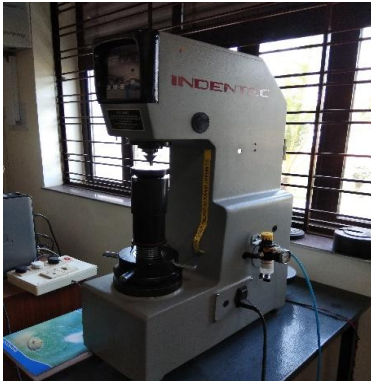
Fig. 3. Details of Brinell's hardness testing machine.
