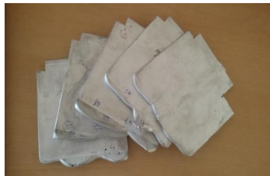
Fig. 2. Cast specimens produced from pit furnace.
