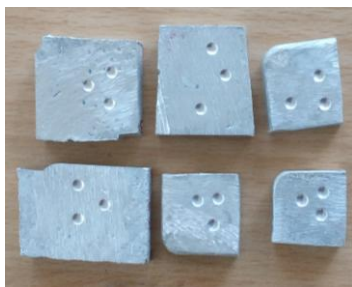
Fig. 4. Details of the indentations at three locations of ball in hardness test specimens.
